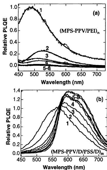
Figure 2 PLQE spectra for (MPS-PPV/PEI)<sub>n</sub> (a) and (MPS-PPV/D/PSS/D)<sub>m</sub> (b)
