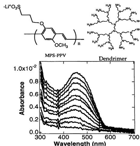
Figure 1 Linear absorption spectra for MPS-PPV/dendrimer multilayer as increasing number of layers
