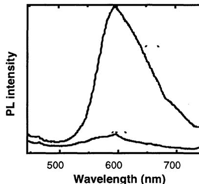
Figure 3 PL of MPS-PPV/dendrimer film (a) with C<sub>60</sub> top layer (b).
