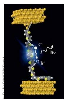
→ Artist's rendering of the electroluminescence of a single molecular polythiophene wire suspended between the tip and the surface of a scanning tunneling microscope.
